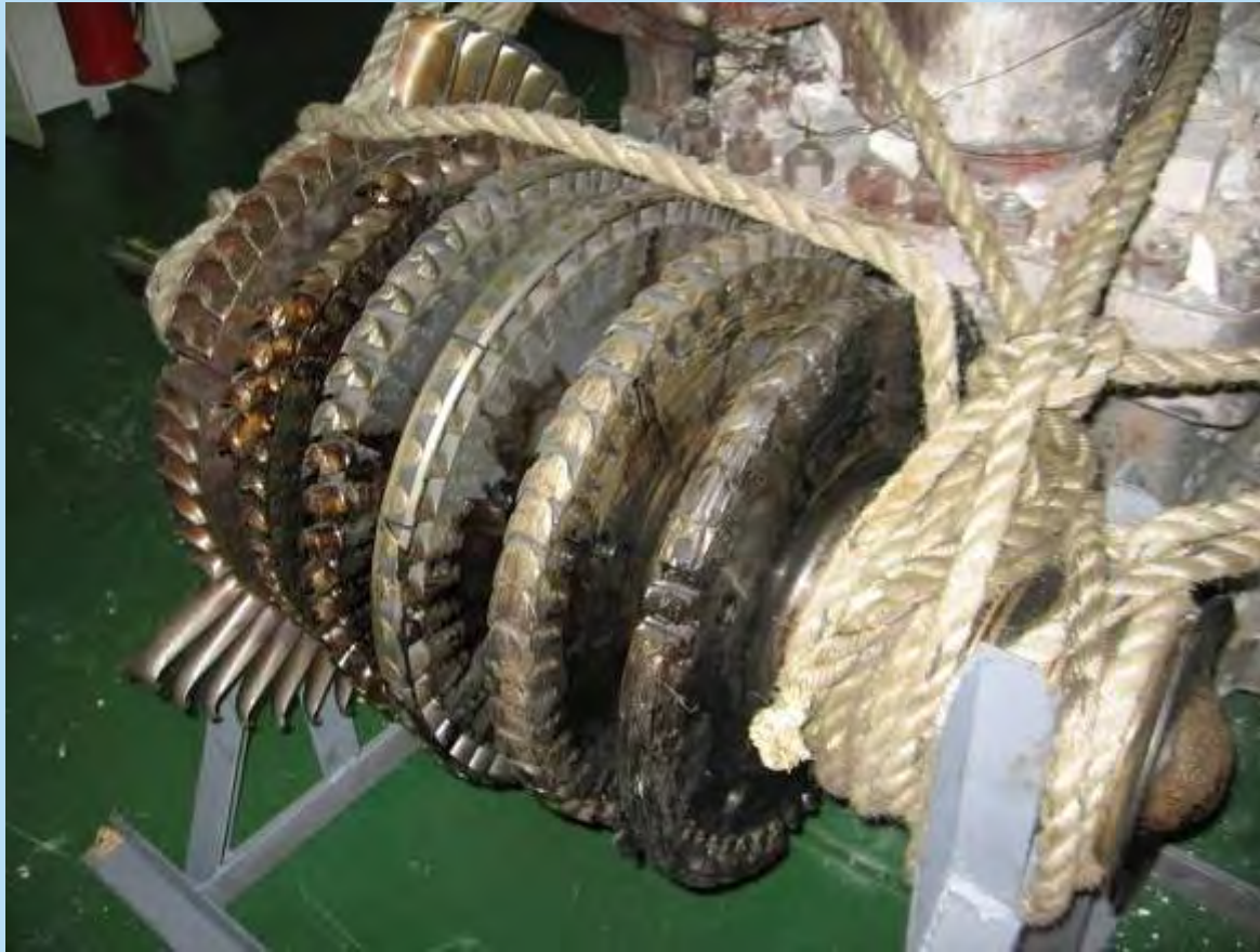
Smashed up steam turbine rotor assembly
